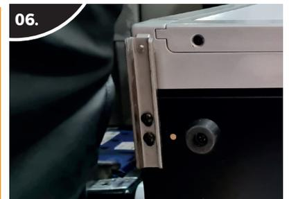
Remove the two screws on the left side of the fridge.
