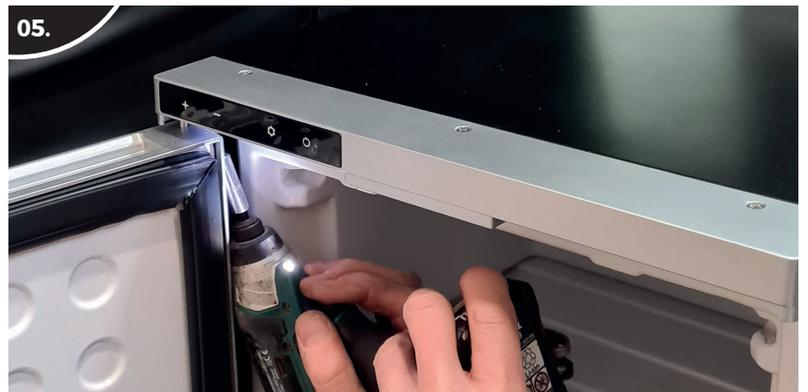
05. Now Refit the Top display panel by screwing the 3 top screws in and then the hinge screw underneath.
