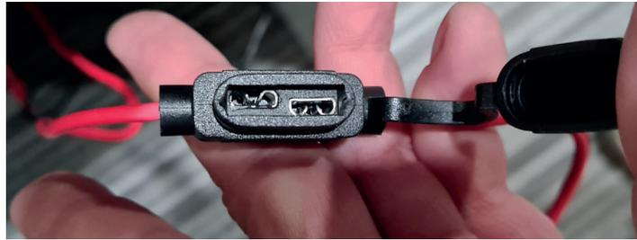
Remove the fuse from the fridge wiring.
