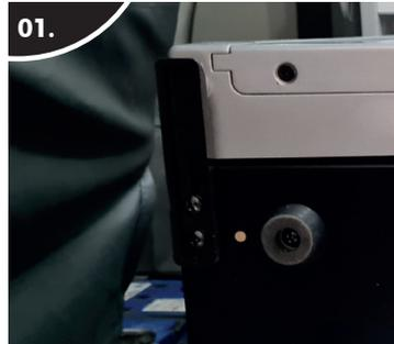
01. Attach the hinge bracket with the two screws to the left hand side of the base of the fridge.
