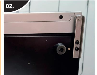
02. Attach the non-hinge bracket with the two screws to the right hand side of the base of the fridge.
