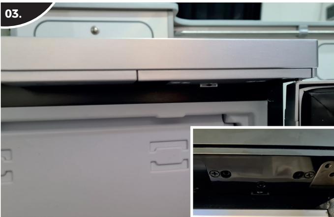
Remove the Blanker on the opposite side of the handle by removing the 3 screws holding the blanker in place from underneath
