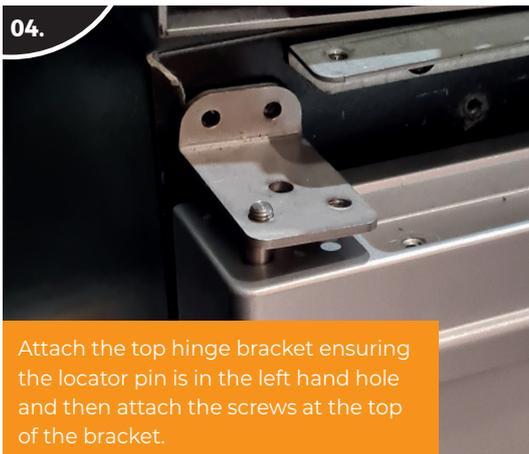
04. Attach the top hinge bracket ensuring the locator pin is in the left hand hole and then attach the screws at the top of the bracket.
