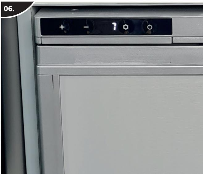
06. Reattach the blanker to the left side beneath the control panel using the 3 screws.
