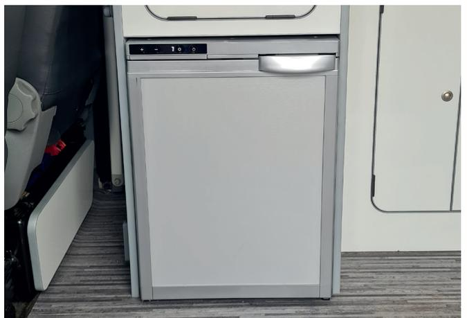
Ensure your JKF50 has been kept upright, on a level surface for 6 hours prior to installation.
